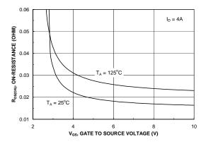
Figure 4. On-Resistance Variation with Gate-to-Source Voltage.
