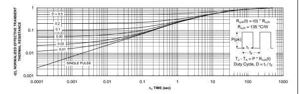
Figure 11. Transient Thermal Response Curve.
