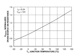
Figure 3. On-Resistance Variation with Temperature.
