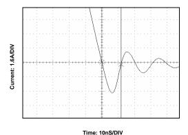
Figure 23. FDS6900AS SyncFET body diode reverse recovery characteristic.
