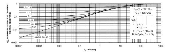
Figure 22. Transient Thermal Response Curve.
