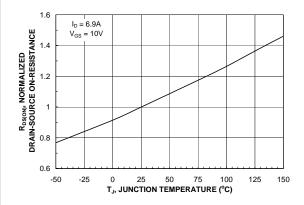
Figure 14. On-Resistance Variation with Temperature.
