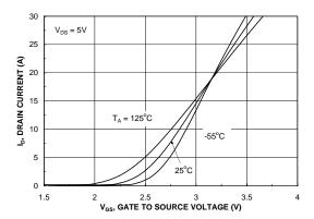
Figure 5. Transfer Characteristics.
