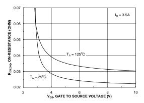
Figure 15. On-Resistance Variation with Gate-to-Source Voltage.
