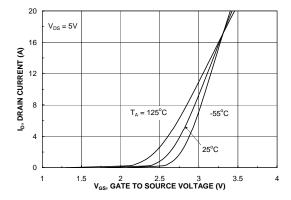
Figure 16. Transfer Characteristics.
