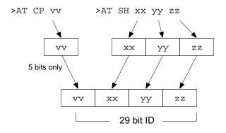
The CAN standard states that for diagnostics, the priority byte ('vv' in the diagram) will always be 18 (it is the default value used by the ELM327). Since it is rarely changed, it can be assigned separately from the other header bytes, using the CP command.
