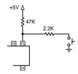
If the circuit is in low power mode, a momentary push of the button will wake it up. This is just one of the many ways in which you can use this input.
