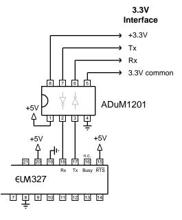
Figure 14. Connecting to a 3.3V System
