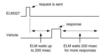
The ELM327 sends a request then waits up to 200 msec for a reply. If none were to come, an internal timer would stop the waiting, and the ELM327 would print 'NO DATA'.
