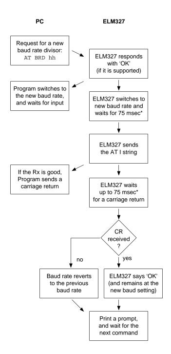
\* the 75 msec time is adjustable with the AT BRT hh command
