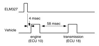
The engine controller responds very quickly, but the transmission takes considerably longer. The adaptive timing algorithm measures the longer transmission response times and will use them to set the timeout, likely to a value in the range of 90 msec. With a timeout of 90 msec, the maximum scan rate would be about 6 readings per second.
