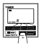
• Change the item setting by pressing keys 1 through 4. (Press the DISPLAY key to switch back from set mode to run mode.)
